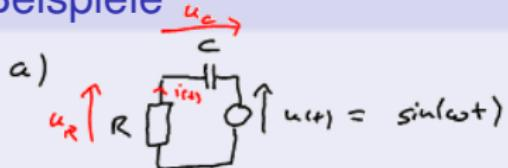
$$\begin{aligned} u(t) &= u_R(t) + u_C(t) \\ \Rightarrow \dot{u}(t) &= \dot{u}_R(t) + \dot{u}_C(t) \\ &= R \dot{i}(t) + \frac{1}{C} i(t) \end{aligned}$$
