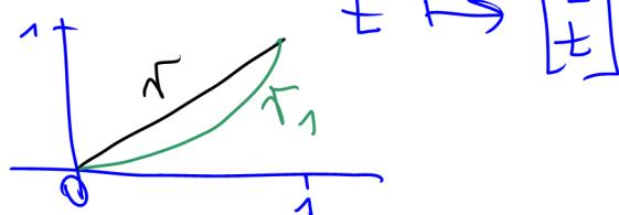
$$\int_{\gamma} F(x) \cdot dx = \int_0^1 \begin{bmatrix} t^3 \\ t^2 \end{bmatrix} \cdot \begin{bmatrix} 1 \\ 1 \end{bmatrix} dt = \int_0^1 t^3 + t^2 dt = \frac{7}{12}$$
